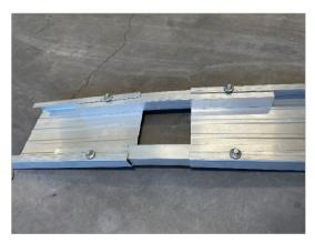
If the connectors are in the base trough, they must be screwed tight with four sheet metal screws.
