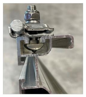
The groove screw of the grounding connector must be screwed into the side groove of the C-N rail. Then insert the earthing wire or earthing cable and tighten the grounding connector. A torque spanner must be used for assembly.
