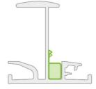
The contact latch must be pressed into the groove of the insertion rail by hand (see picture on the left). The teeth of the contact latch realise the contact with the black anodised aluminium of the module frame.
