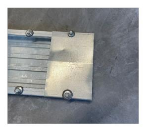
The top cover base trough must be screwed tight with sheet metal screws SW8. If the rail is used as a cable channel, the cable bracket (see step 7) must be inserted before the cover is fitted. The number of the screws per cover must be in proportion to the rail length.
